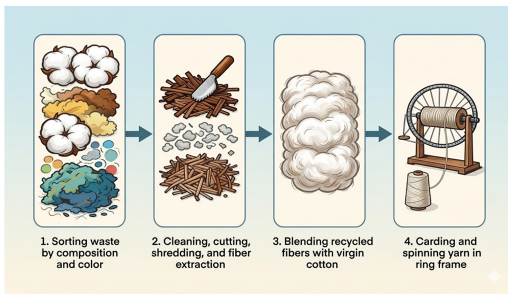
Figure 1. Manufacturing of yarns by blending of virgin and recycled waste.
