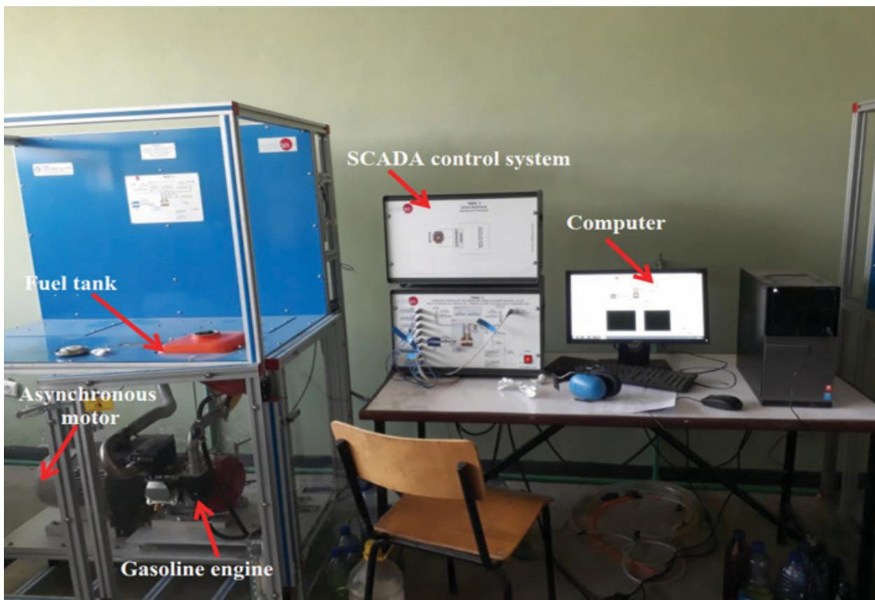
**Figure 1.** Test engine and experimental setup.
