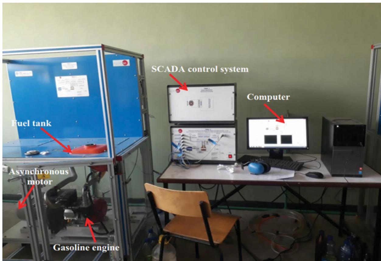
**Figure 1.** Test engine and experimental setup.
