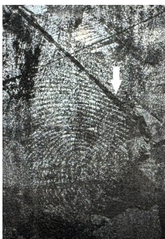
Figure 6. Non-uniform fingerprint development due to scratches on the metal surface (white arrow).
