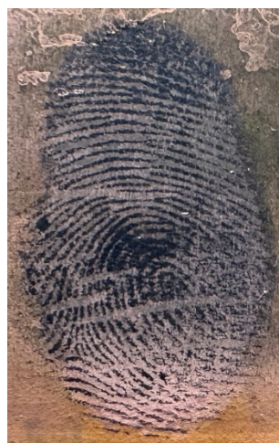
Figure 5. Sebaceous fingerprint deposited on low-carbon steel developed with CuSO 4 solution showing grey ridges and copper valleys.
