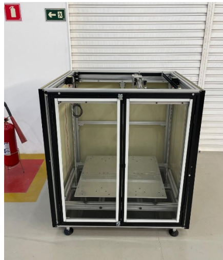
Figure 4. Large scale 3D-printer developed at Federal University of Itajubá used for continuous fiber deposition.
