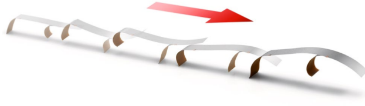
Figure 14. Overlapped images of the mobile robot. The robot consists of the main body and two legs. The materials of the robot are flexible and electrically activated [19].
