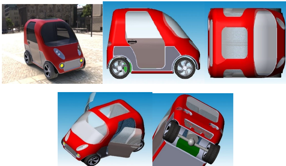
Figure 9. Front, back, top, and side views of a conceptual 3D CAD model of a student-designed electric vehicle (EV) prototype, Features: AGS, self-driving mode, predictive maintenance sensors, solar panel.
