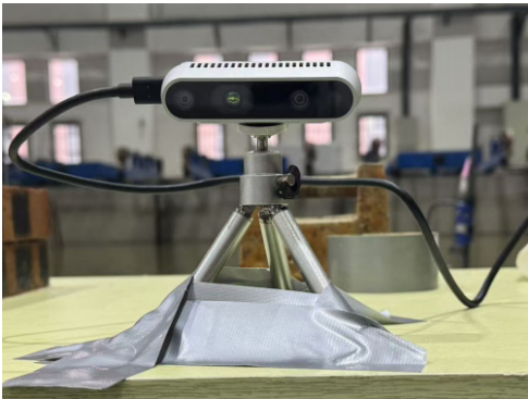
Figure 3. Use of the Intel D325i stereo depth camera in the experiment.
