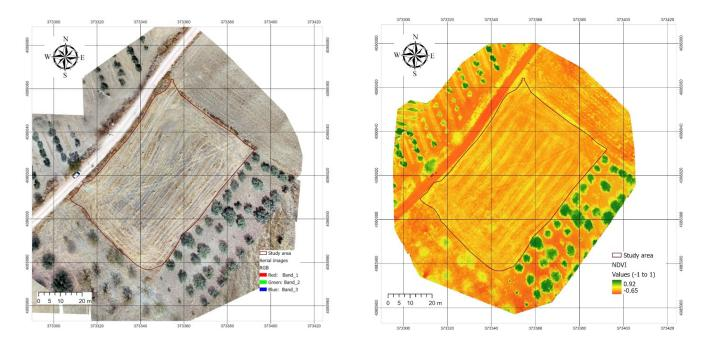
Figure 3. Orthomosaic (left) and NDVI (right) maps.
