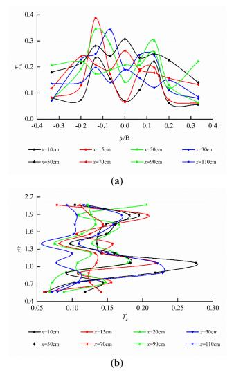
**Figure 12.** Turbulence intensity of egg-shaped orifice (Larger turbulence intensity occurring in the orifice region). (a)  $T_x$  distribution on the horizontal plane at short axis; (b)  $T_z$  distribution on the longitudinal profile at the long axis.
