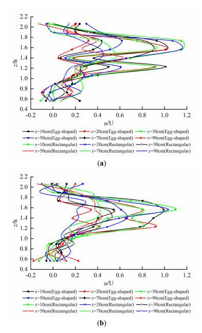
**Figure 9.** Vertical distribution of longitudinal velocity on different longitudinal profiles for egg-shaped and rectangular orifices (The egg-shaped orifice exhibits two peaks, while the rectangular orifice one peak). (a) Vertical distribution of longitudinal velocity on longitudinal profile at the long axis of the orifice; (b) Vertical distribution of longitudinal velocity on longitudinal profile at b/4 of the orifice.
