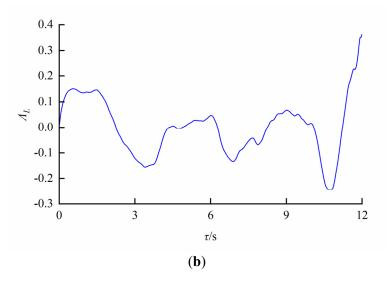
**Figure 18.** Integral scale of turbulence in different regions due to an egg-shaped orifice (Eddies within orifice region vary in integral scale). (a) Orifice region; (b) Non-orifice region.
