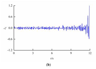
Figure 17. Turbulencemicroscalein different regions due to an egg-shaped orifice (Larger eddy within the orifice region). (a) Orifice region; (b) Non-orifice region.
