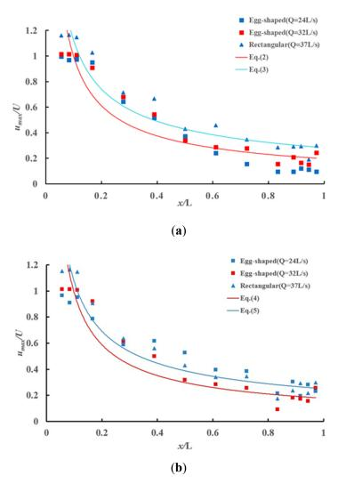
**Figure 5.** Variation in the maximum longitudinal velocity along flow direction for egg-shaped and rectangular orifices. (a) Variation of the maximum longitudinal velocity along flow direction on the horizontal plane (The velocity for the egg-shaped orifice decays more rapidly than that for the rectangular one); (b) Variation of the maximum longitudinal velocity along flow direction on the longitudinal profile.
