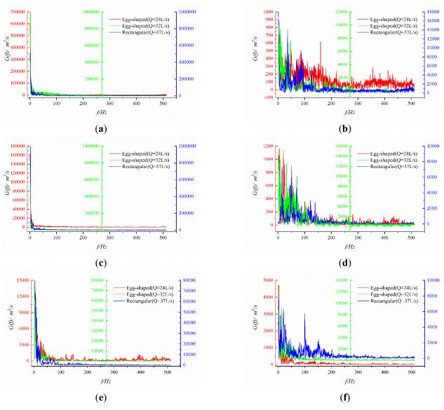
**Figure 20.** Spectral characteristics of velocity fluctuations at different points for egg-shaped and rectangular orifices. (a) Longitudinal velocity fluctuation (x/L = 0.28); (b) Transverse velocity fluctuation (x/L = 0.28); (c) Longitudinal velocity fluctuation (x/L = 0.39); (d) Transverse velocity fluctuation (x/L = 0.39); (e) Longitudinal velocity fluctuation (x/L = 0.50); (f) Transverse velocity fluctuation (x/L = 0.50).
