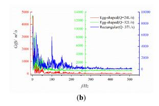
**Figure 19.** Spectral characteristics of velocity fluctuation at specific points (x/L = 0.50) for egg-shaped and rectangular orifices. (a) Longitudinal velocity fluctuation; (b) Transverse velocity fluctuation.
