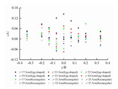
**Figure 10.** Transverse distribution of transverse velocity on cross section at x/e = 15 for egg-shaped and rectangular orifices (Exhibiting upward convex in the lower semi-ellipse, and downward concave in the upper semi-circle for egg-shaped orifice, and less fluctuation for rectangular one).
