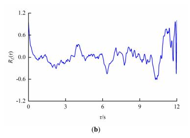
Figure 16. Auto-correlation coefficient of velocity fluctuation in different regions of egg-shaped orifice (Shorter cycle and lower amplitude). (a) Orifice region; (b) Non-orifice region.
