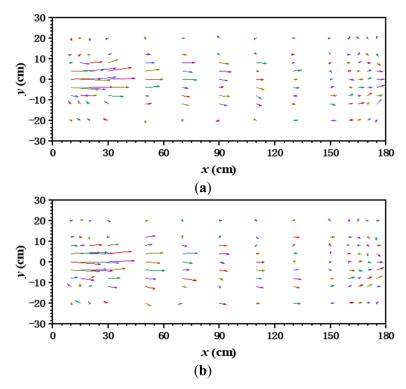
**Figure 3.** Velocity vector on different horizontal planes of egg-shaped orifice (The jet issues from the left end). (a) Horizontal plane at the focus of lower semi-ellipse; (b) Horizontal plane at the short axis of the lower semi-ellipse.
