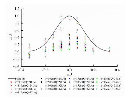
**Figure 6.** Transverse distribution of longitudinal velocity on the horizontal plane at the short axis of the egg-shaped orifice (It is considerably characterized by three-dimensionality, apparently different from a plane jet).
