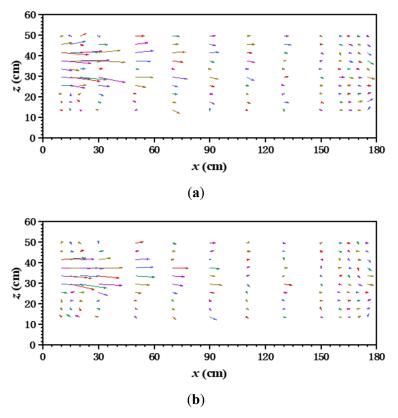
**Figure 4.** Velocity vector on different longitudinal profiles of egg-shaped orifice (The jet issues from the left end). (a) Longitudinal profile at the long axis of the lower semi-ellipse; (b) Longitudinal profile at 3b/4.
