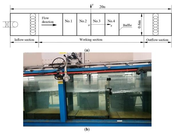
Figure 1. Fishway flume. (a) Plan view of fishway flume; (b) Experimental setup of fishway flume.
