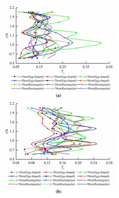
**Figure 14.**  $T_z$  distribution on different longitudinal profiles for egg-shaped and rectangular orifices (Saddle-shaped distribution for egg-shaped orifice, and multiple peaks for rectangular one). (a)  $T_z$  distribution on the longitudinal profile at long axis of orifice; (b)  $T_z$  distribution on the longitudinal profile at b/4 of the orifice.
