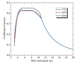
Figure 11. Blade power coefficient with different wind speed.
