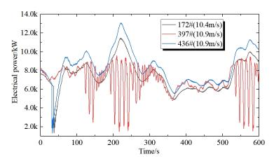
Figure 17. Electrical power under rated operating conditions.
