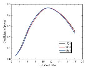
Figure 10. Blade power coefficient with different tip speed ratio.
