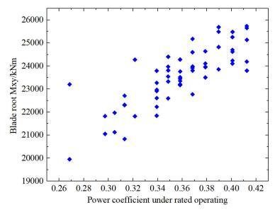
Figure 8. Blade power coefficient with different root load.
