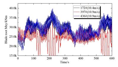
Figure 18. Root load (Mxy) under rated operating conditions.
