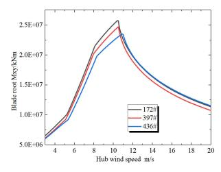
Figure 15. Root load with different blades.
