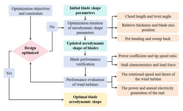
Figure 1. Functional diagram of optimization design method.
