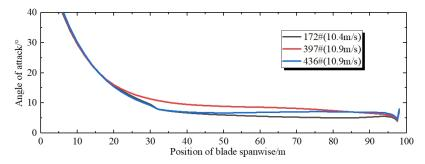
Figure 19. Attack angle distribution under rated operating conditions.
