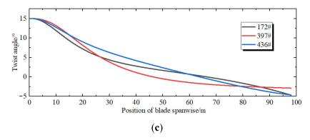
Figure 9. Aerodynamic shape of the optimized blade. (a) Chord length; (b) Relative thickness; (c) Twist angle.
