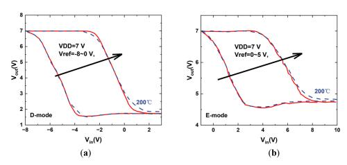
**Figure 20.** DC output characteristics of GaN comparators by (a) D-mode (b) E-mode differential pairs at 200 °C, respectively (created by the authors based on [98]).
