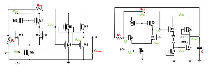
Figure 21. Circuit schematic diagram of the sawtooth waveform generator, (a) [97] and (b) (created by the authors based on [96]).
