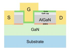
Figure 12. Schematic cross-section of the GaN MOS-HEMT.
