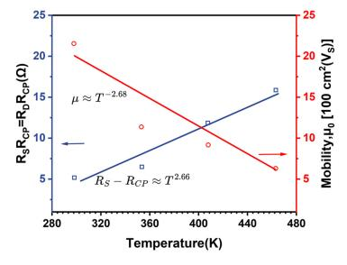
**Figure 6.** Temperature dependence of  $\mu_0$ , ungated 2-DEG resistance  $R_{S-}R_{CP} = R_D - R_{CP}$  at  $V_{GS} = -4$ V and  $\mu_{s0}$  (created by the authors based on [29]).
