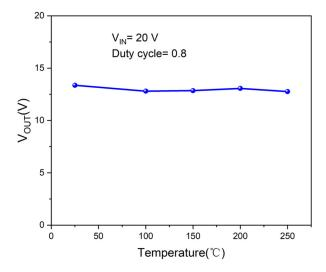
Figure 28. Experiments results of synchronous converter at various tempetatures and duty cycles (created by the authors based on [110]).
