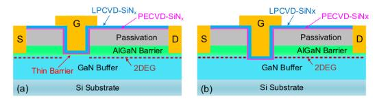
Figure 4. (a) MIS-HEMT with partially recessed-gate structure and (b) MIS-FET with fully recessed-gate structure [25].
