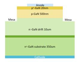
Figure 11. Schematic cross-section of the GaN PIN diode (created by the authors based on [47]).
