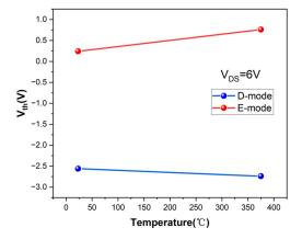
Figure 1. Characteristics of D-mode HEMTs and E-mode HEMTs at different temperatures (created by the authors based on [12]).
