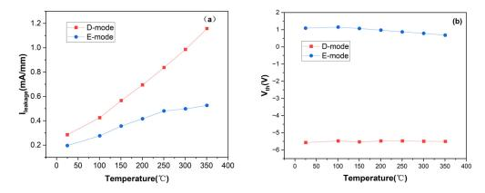
Figure 2. The temperature dependence of off-state drain leakage current ( $I_{leak}$ ) (a) and  $V_{th}$  (b) for E/D-mode GaN HEMTs by the planar process (created by the authors based on [15]).
