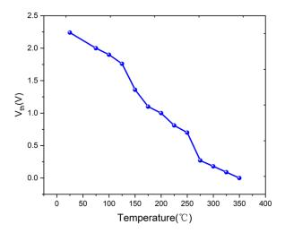
Figure 25. The V<sub>th</sub> drift of recessed gate GaN inverters at 25–350 °C (created by the authors based on [101]).
