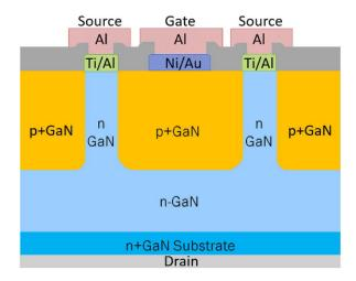
Figure 10. Schematic cross-section of the fabricated vertical GaN Fin-JFET [46].
