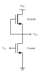
Figure 22. GaN inverter circuit schematic diagram.
