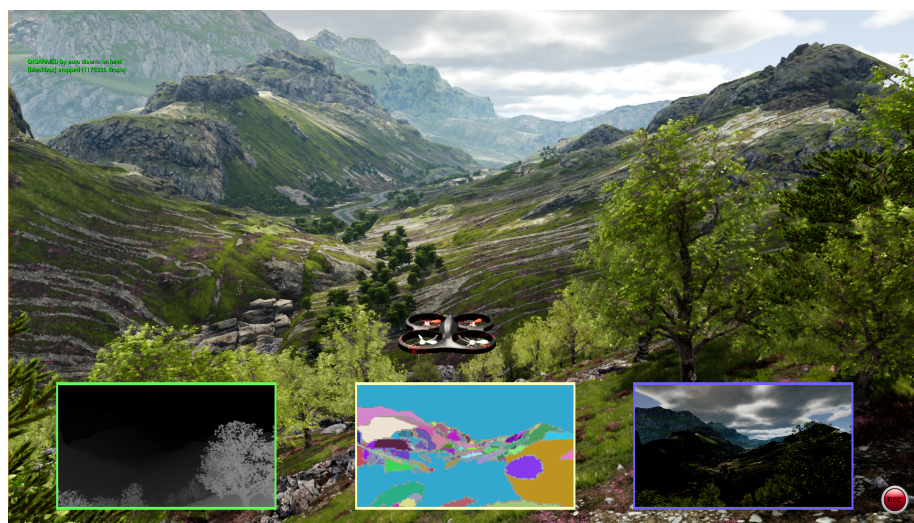
Figure 3. Example of a high-fidelity drone simulation environment using AirSim simulator (© Microsoft Corporation, released under the MIT License).
