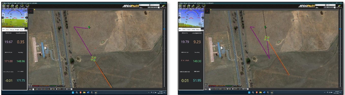
Figure 8. The Flight Path Traced by the Drone: flying towards Waypoint 2 and Returning to Launch on the left and right panels, respectively.
