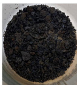
a) Compressor cartridge Organic soluble 14% HCl soluble 56% Residue 25%
