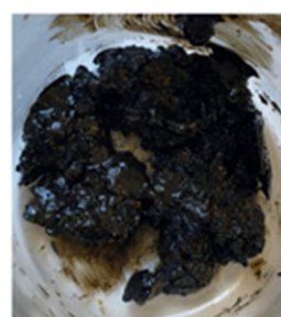
b) Compressor diaphragm Organic soluble 40% HCl soluble 38% Residue 18%
