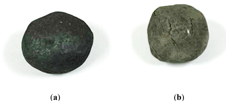
Figure 1. Samples used in the experiment, (a) pellets; (b) DRI.
