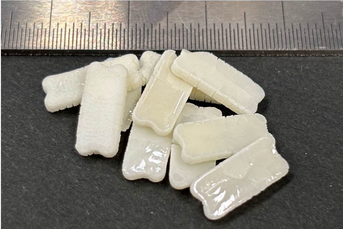
Figure 4. Monolithic TiO 2 ceramic photocatalyst.
