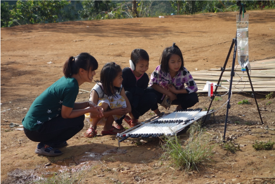
Figure 8. The trial of the solar water purification system in Chiang Rai Province, Thailand (Length of photocatalyst tube = 13 m) (Photo: Negishi).
