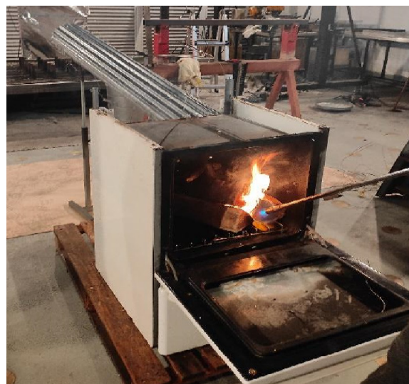
Figure 3. Igniting the fire in the converted oven for test 3.
