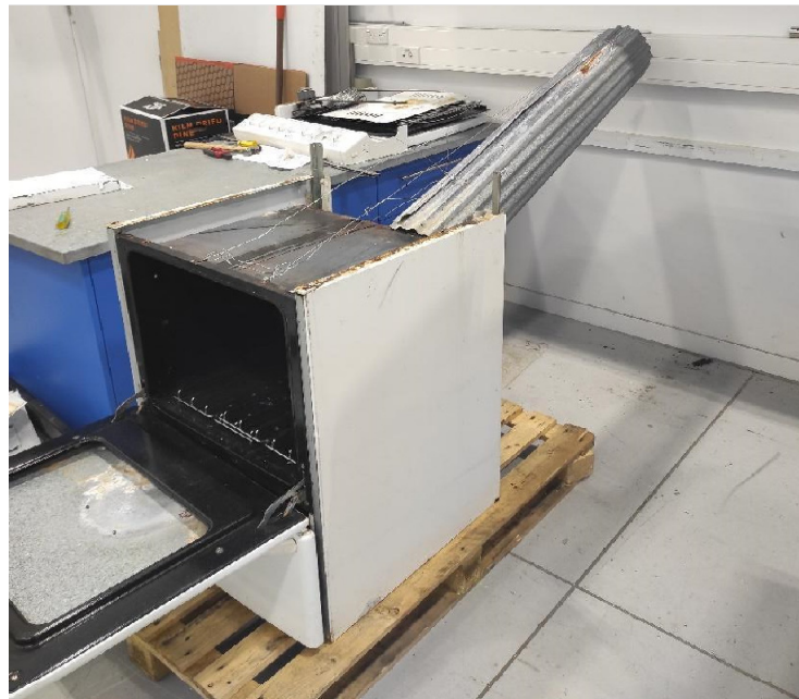
Figure 2. Photograph of the repurposed oven, showing the door opening, sheet metal chimney, and door with the inner glass pane replaced with sheet metal.
