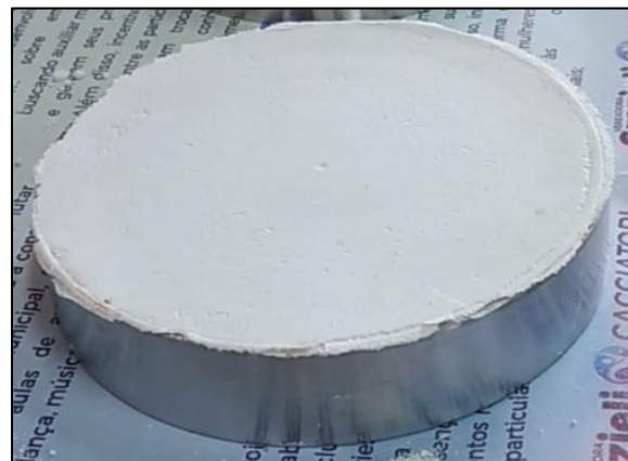
Figure 7. Irregularities on the surface of compacted BaSO 4 .
