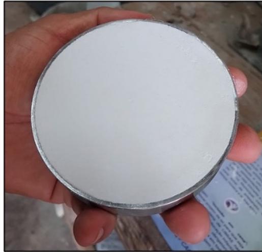
Figure 8. Irregularities on the BaSO 4 surface removed with 2000 and 3000 grit water sandpaper.
