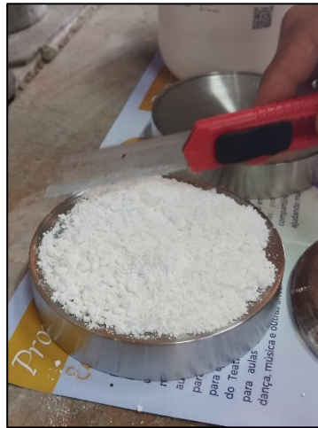
Figure 5. Stainless steel part filled with BaSO 4 .
