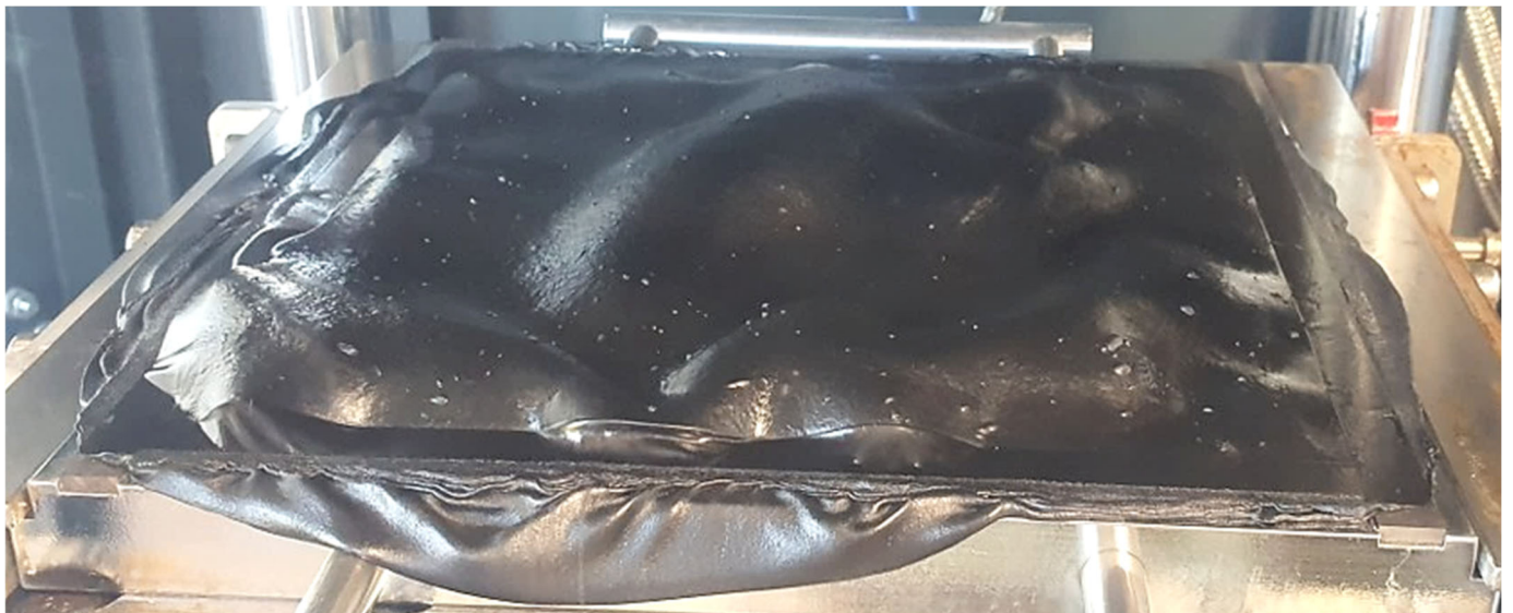
Figure 2. Photo of the vulcanized IIR compound with BG material as filler (1 mm sheet thickness with blistering).
