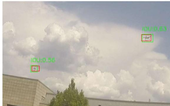
**Figure 3.** IoU results, where the green bounding boxes represent ground truth, and the red boxes indicate the predictions.
