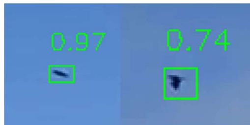
**Figure 7.** Examples of birds are incorrectly identified as drones due to similar visual patterns and size.
