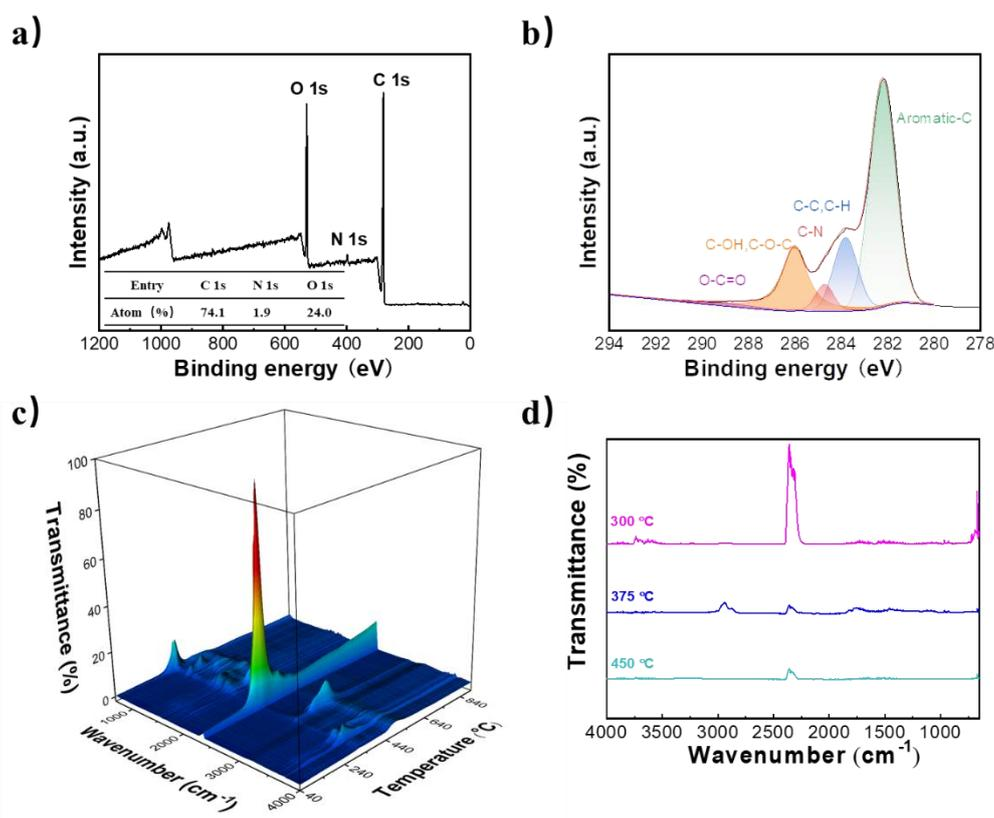
**Figure 6.** (a) Wide-scan XPS spectrum; (b) C1s XPS spectrum of ER08-60 coke residue; (c) 3D TG-IR spectra of the degradation component in gas phase; and (d) FT-IR spectra of the pyrolysis for ER08-60.
