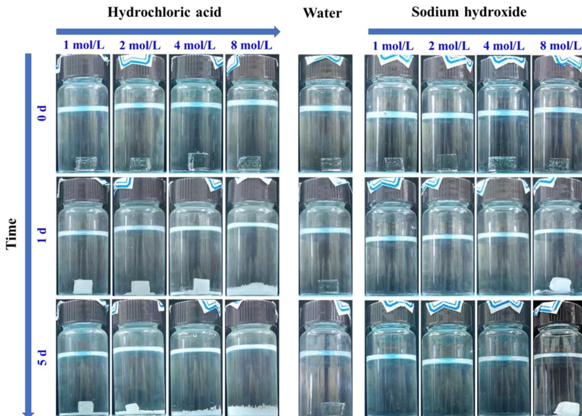
**Figure 7.** Photo images of ER08-60 hydrolyzation samples in acidic, neutral and basic solutions.
