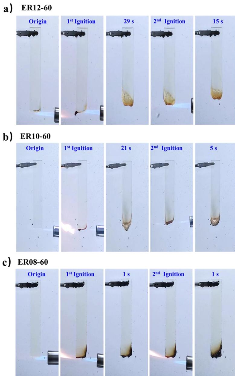
**Figure 3.** The video screenshots of samples (a) ER12-60; (b) ER10-60 and (c) ER08-60 during vertical burning (UL-94) tests.
