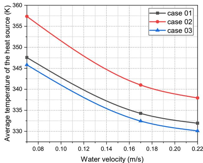
**Figure 8.** The variation of average temperature of the heat source vs. water velocity.
