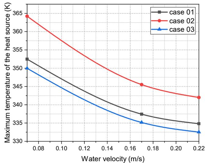
**Figure 7.** The variation of maximum temperature of the heat source vs. water velocity.
