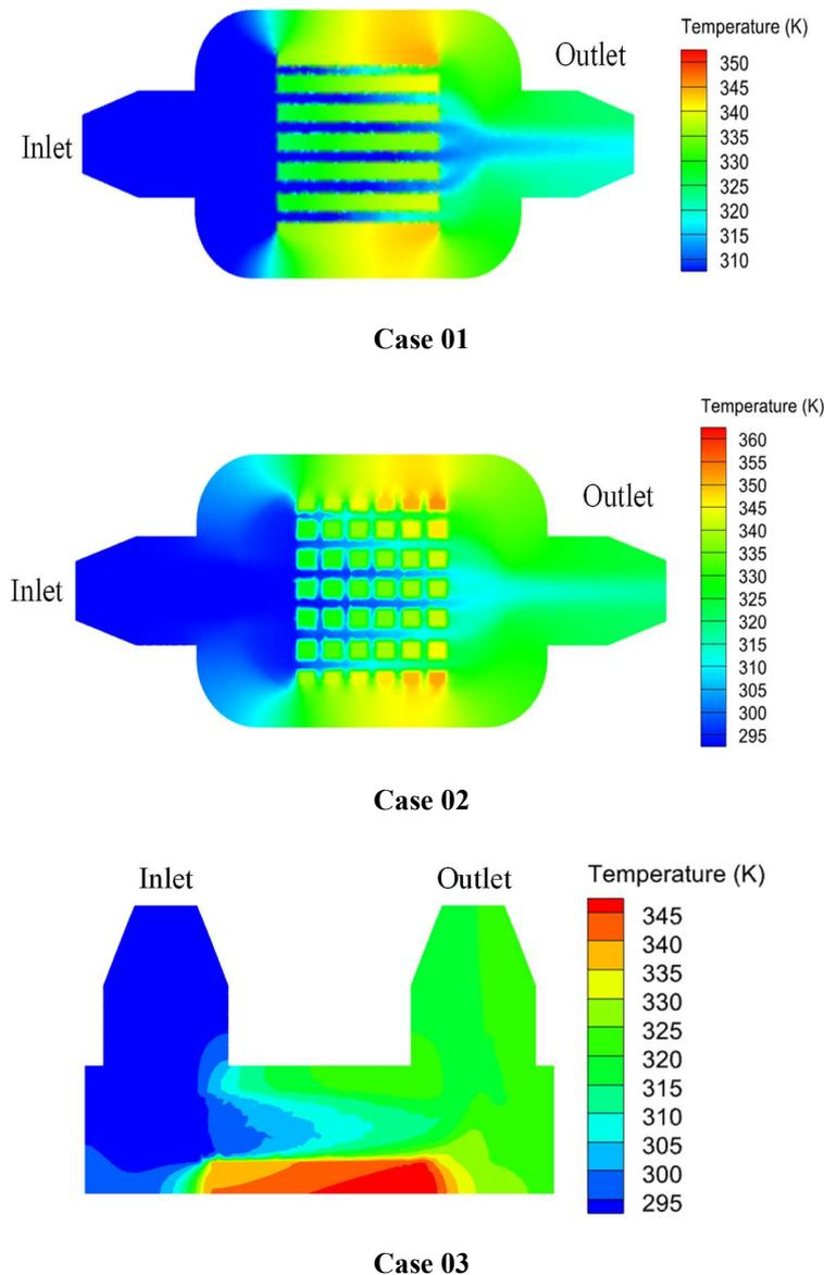
**Figure 6.** The temperature distribution for three cases at a level equal to 0.011 m from the bottom of the heat sink.
