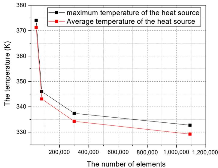
**Figure 3.** The effect of the elements number on the temperature results for case 01. (flow rate = 0.17 m/s).
