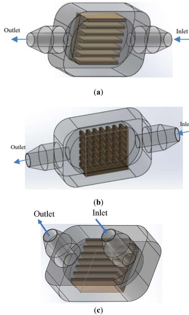
**Figure 1.** Shapes geometric studied. **(a)** case 01: Rectangular-channel heat sink featuring a horizontal inlet and outlet; **(b)** case 02: The mini pin fin heat sink with a horizontal inlet and outlet; **(c)** case 03: Rectangular-channel heat sink featuring a vertical inlet and outlet.
