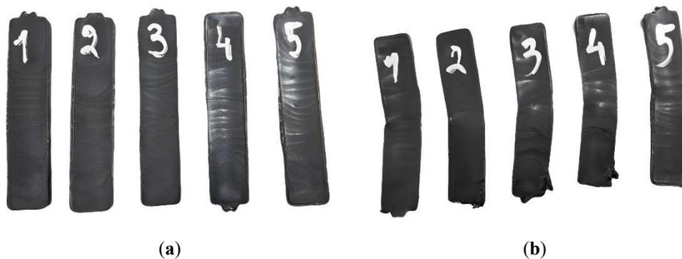
**Figure 1.** Unnotched impact test specimen. (a) Sample before testing; (b) Sample after testing.
