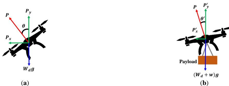
**Figure 2.** Forces on a drone with payload. (a) A drone without on-board payload; (b) A drone with payload  $w$ .
