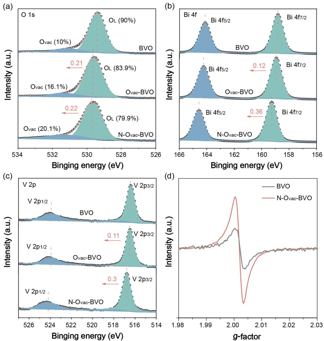
**Figure 2.** (a) O 1s, (b) Bi 4f, and (c) V 2p XPS spectra of BVO, N-O<sub>vac</sub>-BVO and N-O<sub>vac</sub>-BVO photoanodes. (d) EPR spectra of BVO and N-O<sub>vac</sub>-BVO photoanodes.
