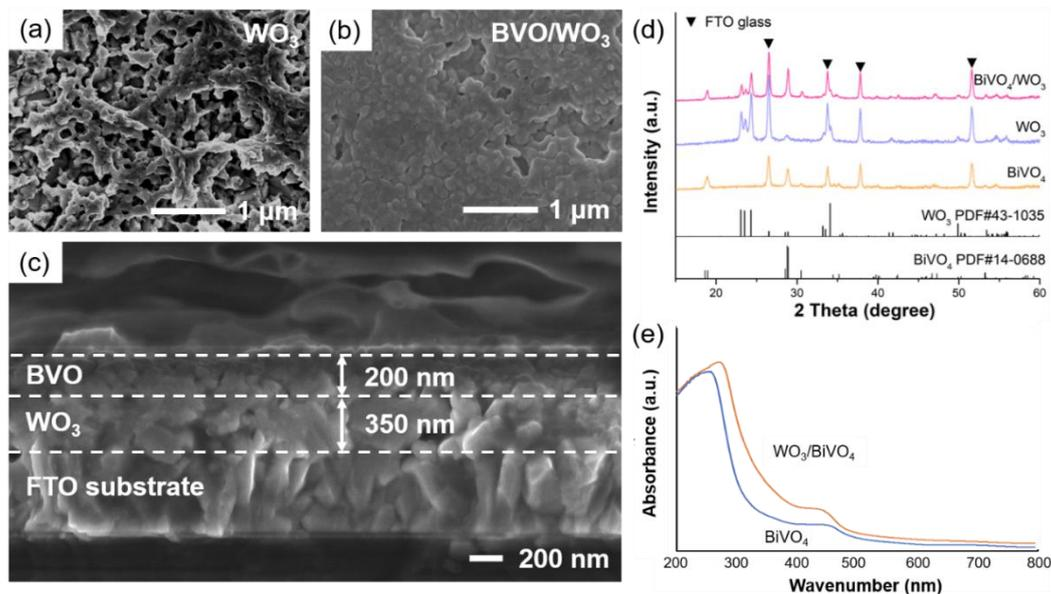
**Figure 1.** Top-view SEM images of (a) WO<sub>3</sub> and (b) WO<sub>3</sub>/BVO photoanodes. (c) Cross-sectional SEM photograph of WO<sub>3</sub>/BVO photoanode. (d) XRD analysis of WO<sub>3</sub>, BVO, and WO<sub>3</sub>/BVO photoanodes. (e) UV-Vis spectrum of WO<sub>3</sub>/BVO photoanode.
