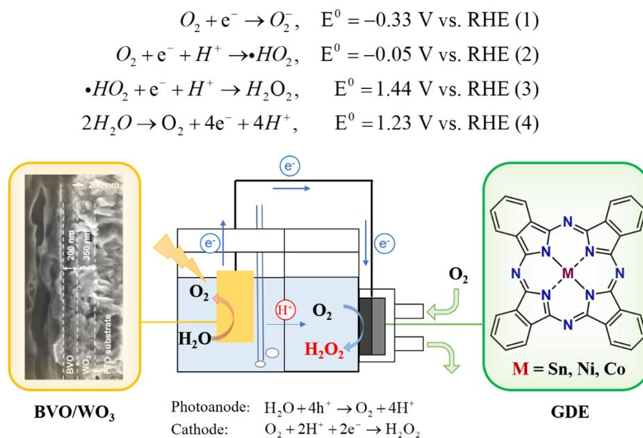
**Scheme 1.** A tandem electrode strategy for the synthesis of H<sub>2</sub>O<sub>2</sub>.
