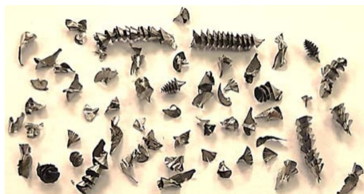
Figure 5. Chip morphology after UVAM [46].
