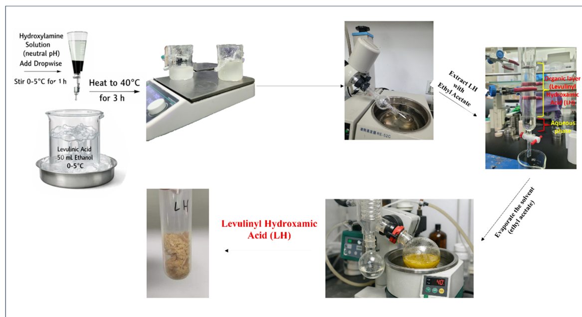
Figure 1. Schematic representation of the synthesis of levulinyl hydroxamic acid (LH), showing the low-temperature hydroxylamine addition, controlled heating, liquid-liquid extraction, and solvent evaporation sequences used to obtain the isolated product of LH.
