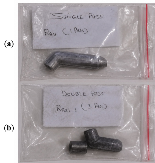
Figure 11. Single pass and double pass ECAP processing specimen. (a) Single Pass; (b) Double Pass.
