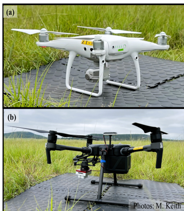
Figure 3. (a) The DJI Phantom 4 Pro (20MP CMOS sensor) was used for the colour imagery. (b) The DJI Matrice 210 (20MP CMOS sensor) with a Micasense RedEdge-MX multispectral sensor was used for multispectral imagery.
