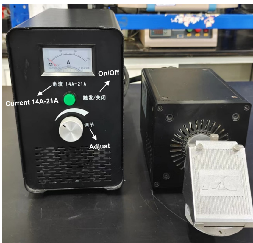
Figure S1. The xenon lamp light source system.
