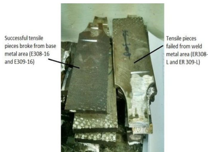
Figure 8. Fractured samples of SMAW (at left ) and TIG welding (at right ) after tensile testing.
