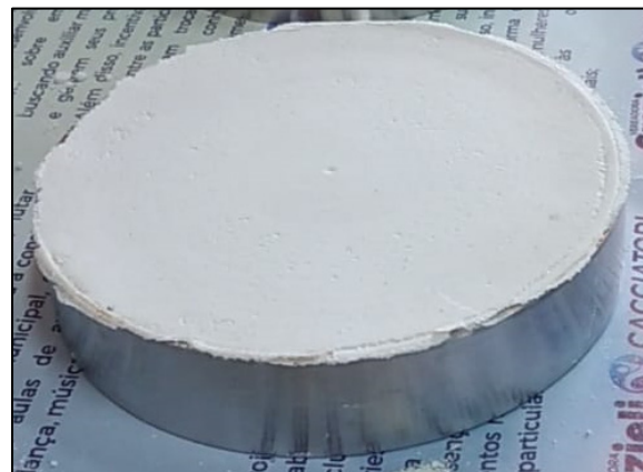
Figure 7. Irregularities on the surface of compacted BaSO 4 .
