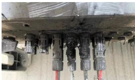
Figure 2. Arc fault of PV connectors.
