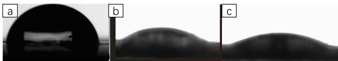
Figure 9. The water contact angle of the (a) PI, and polyimide membranes: (b) electrostatic porous and (c) template method.
