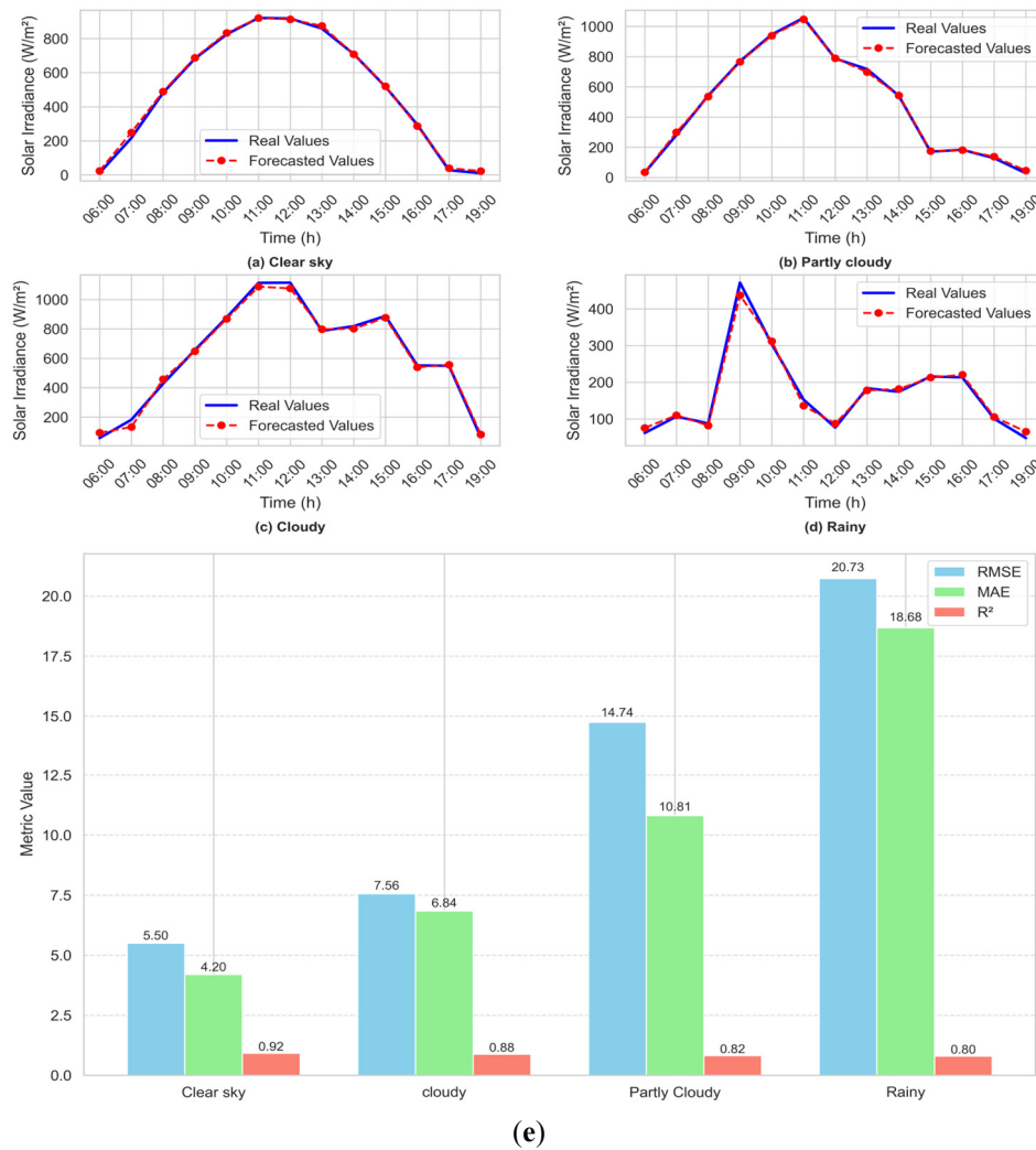
Figure 7. Comparison of real and forecasted solar irradiance values under different weather conditions: (a) clear sky, (b) cloudy, (c) partly cloudy, and (d) rainy conditions; (e) comparison of statistical performance metrics (MAE, RMSE, and R^2 ).
