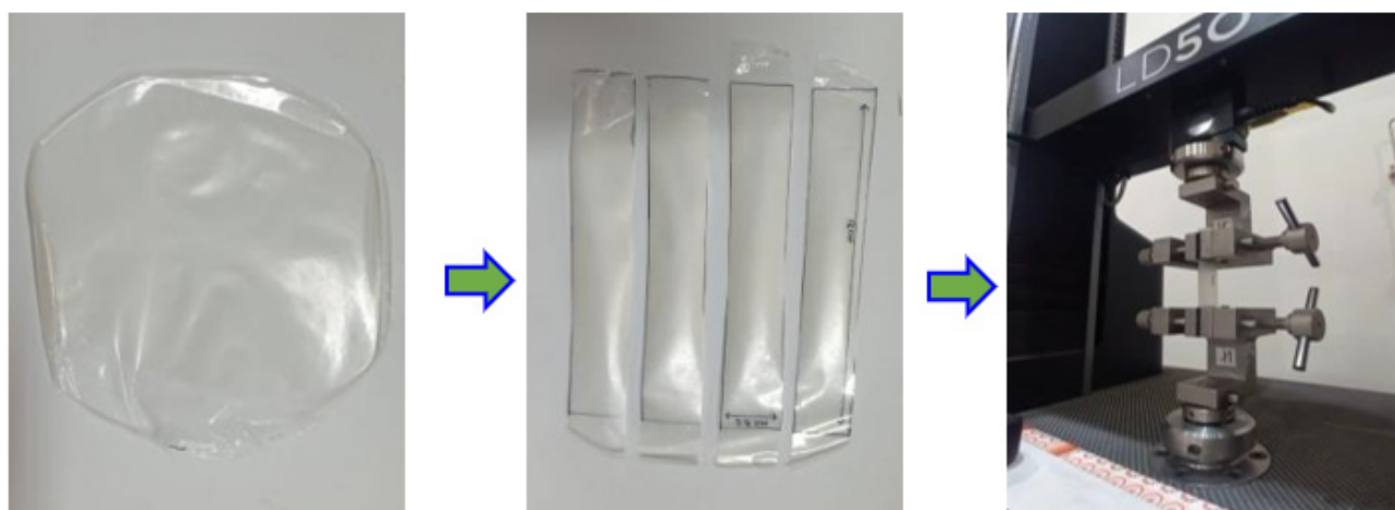
Figure 4. Tensile Testing of Nitrocellulose Film.
