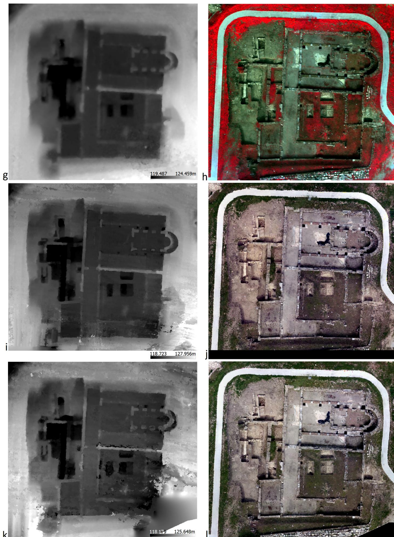
Figure 8. (g) DSM and (h) MS orthophoto mosaic (bands: G, R, NIR) of Sequoia+, 45 m flight height; (i) DSM and (j) RGB orthophoto mosaic of Sequoia+, 30m flight height; (k) DSM and (l) RGB orthophoto mosaic of Sequoia+, 45m flight height.
